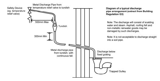
General guidance is provide by the above diagram extracted from the G3 Building Regulation Guidance. This guidance is available as a free of charge download of the G3 Approved Document from www.planningportal.gov.uk. The discharge from both the temperature relief and expansion relief valves can be joined together via a 15mm end feed tee.
